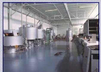
**General Characteristics:** Light stable, high-gloss or satin finish provides light reflectivity. Resists staining and minor chemical spills of cleaning and industrial chemicals. Provides a "Breathable" coating to allow transmission of moisture through the coating without failure. 10 Perms @ 5 mils DFT. Designed for use as a decorative floor finish. Complies with VOC regulations for Industrial Maintenance Coatings in the OTC and CA
