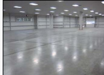
**General Characteristics:** Low Odor, High chemical resistance, Excellent impact and abrasion resistance, Flexible, 600% elongation, Remains flexible, Resists hot water dumping up to 250°F, Resists staining and major chemical spills of cleaning and industrial chemicals, Meets USDA requirements, Complies with VOC regulations for Industrial Maintenance Coatings in the OTC and CA.
