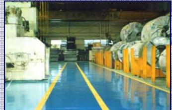
**General Characteristics:** Light stable, high-gloss finish provides light reflectivity. Resists Skydrol®, jet fuels and other industrial chemicals. Provides a high degree of resistance to tire staining. Designed to withstand industrial traffic. Complies with VOC regulations for Industrial Maintenance Coatings in OTC & CA\* (\*excluding SCAQMD).
